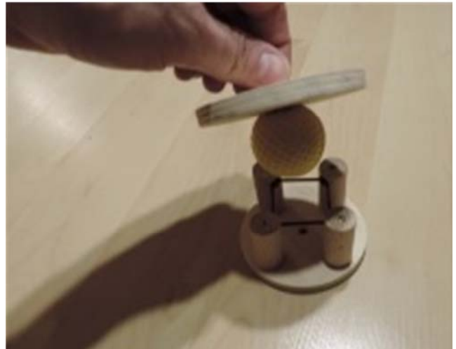
Figure 5. Bolt hook in a rawl plug – the screw causes the plastic rawl plug to expand radially outwards.
